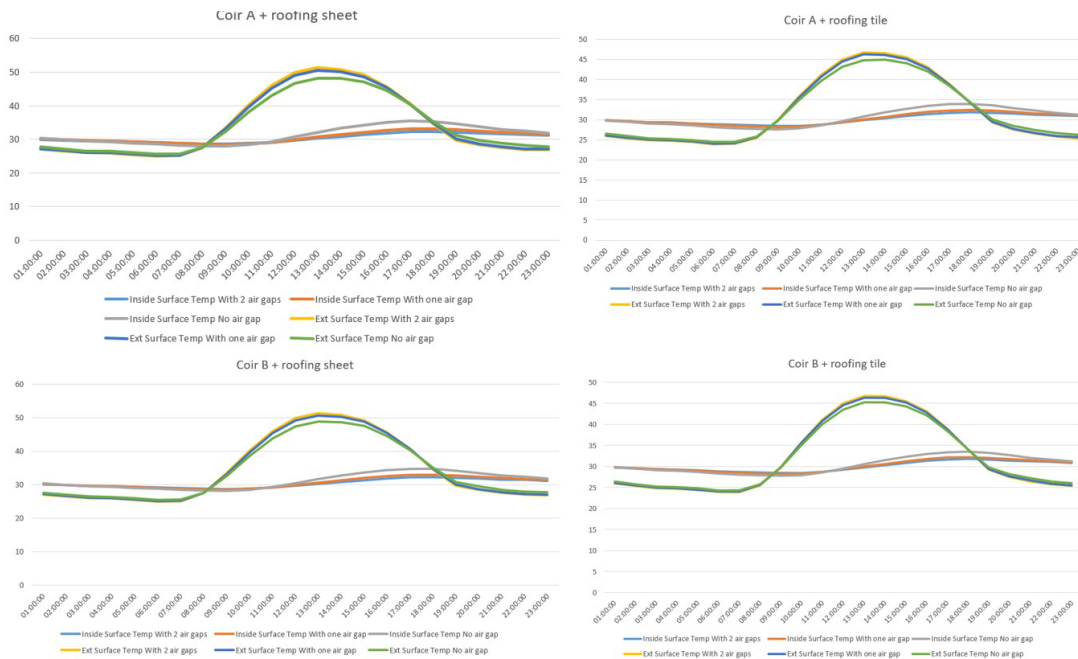
Figure 15: Comparison between T_{si} and T_{so} for each design case based on variation in presence of air gap. Source: Author
