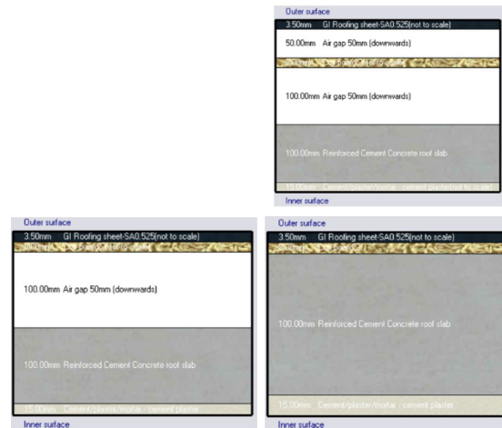
Figure 13: The 3 cases of air gaps: (i) Presence of 2 air gaps, (ii) Presence of 1 air gap, (iii) No air gap. Source: Author
