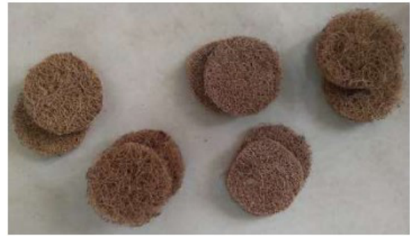
Figure 5: Samples prepared in circles. Source: Coir Board, 2022
