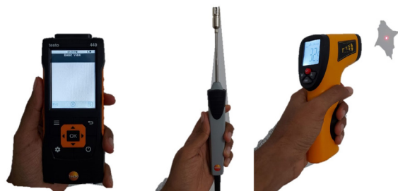
Figure 2: Testo440; Controller(left), Thermocouple probe(middle) & MCP; Infrared thermometer gun(right), Source: Photographed by author
